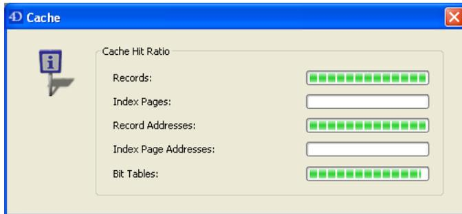
This window provides additional thermometers indicating how the cache is being used. For each type of data that can be kept in the cache, there is a thermometer indicating how much of the data is present in the cache. A higher reading is considered advantageous, because accessing that type of data will require fewer occurrences of disk access (hits).
